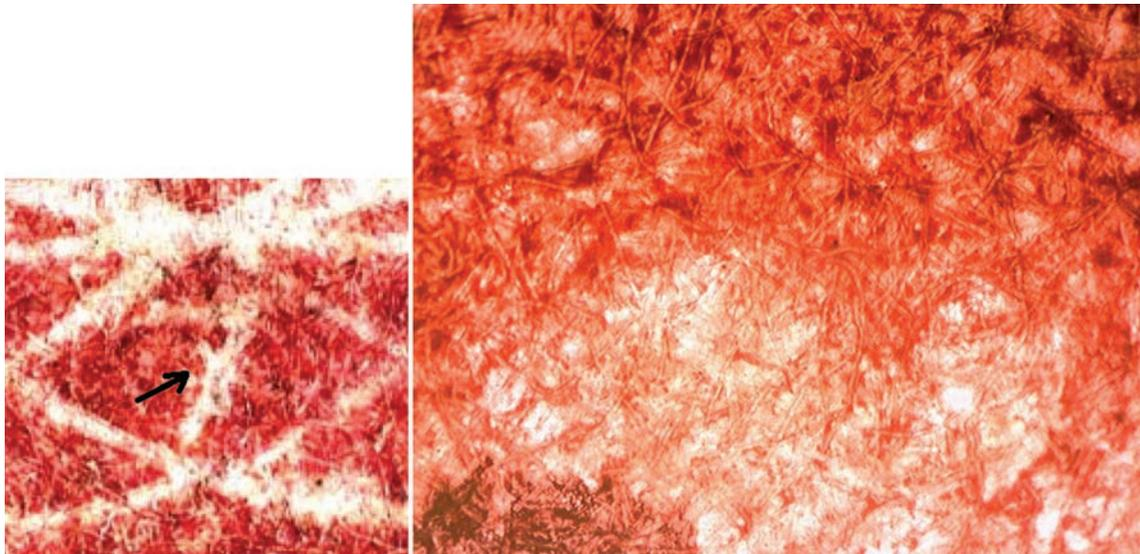
FIGURE 18. The image on the right is a  $\times 100$  enlargement of a small area (left, black arrow) from the top of the right-hand “7” of the SK stamp from the Victor Hugo cover. The general matted appearance of the paper fibers at this magnification is clearly visible, and any fiber disturbance would also be visible under this magnification.
