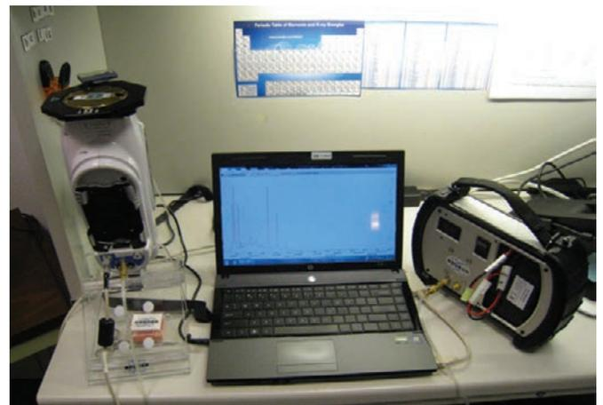
FIGURE 6. Bruker Tracer III-SD X-Ray Fluorescence Analyzer.
