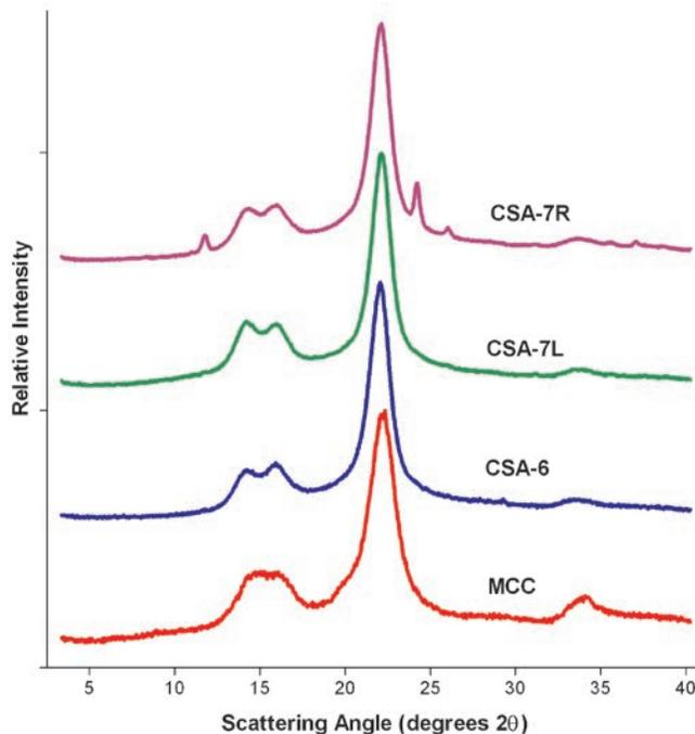
FIGURE 7. X-ray diffraction patterns of microcrystalline cellulose and the corresponding patterns obtained on the faces of the reference stamps. Image used with the permission of *The Confederate Philatelist*.
