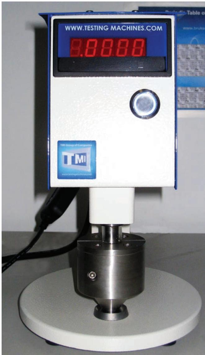
FIGURE 4. Testing Machines Inc. model 49-76-01 micrometer.
