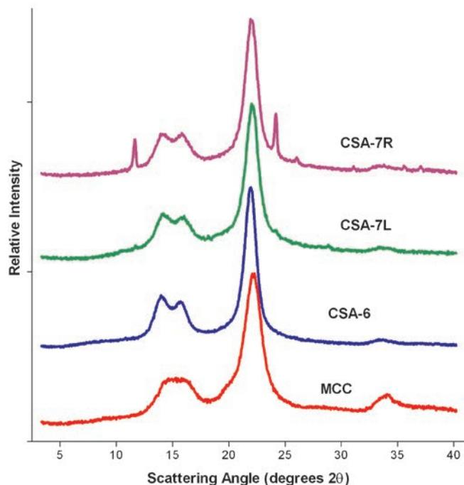
FIGURE 5. X-ray diffraction patterns of microcrystalline cellulose and the corresponding patterns obtained on the margins of the reference stamps. Image used with the permission of *The Confederate Philatelist*.
