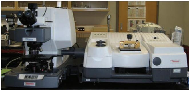
FIGURE 9. Thermo Nicolet FT-IR with Continuum microscope.
