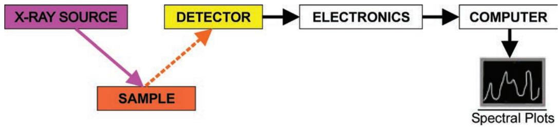
FIGURE 6. An example of a drawing or sketch used to provide a simple description of a possibly complex process. This is the logical design of an EDXRF spectrometer.
