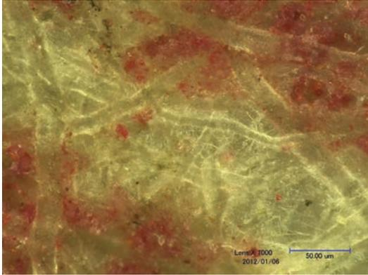
**FIGURE 14.** Depth composition analysis of the top of the right-hand “7” from stamp SL from the Victor Hugo cover. Such a recess of a colorless area can be produced only through impact between the plate and the paper at the time of printing and cannot be produced through faking.
